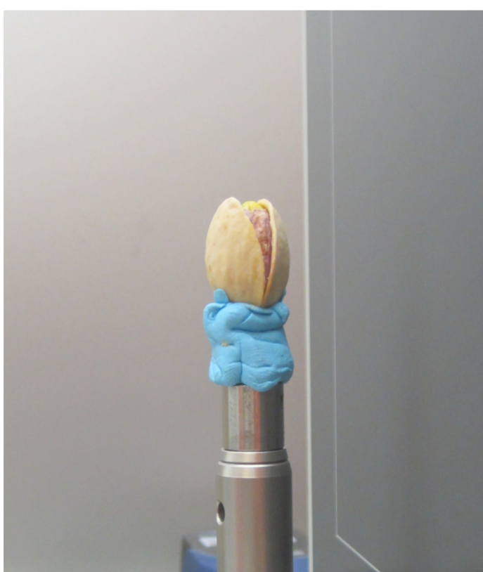
Figure 1: Picture of the target ready for imaging. Size of nut: 1,9 cm long and 1,4 cm wide.
