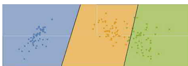
Figure 6.9: An example of a heuristic classification of the Iris data (after the LDA transform) and the resulting areas of the variable space for the three classes.
