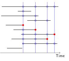
Follow-up data with 10 observations and 4 observed failure times. At each observed failure time •
