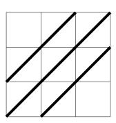
Give a numbering to the nine pixels  $(f \in \mathbb{R}^9)$  and to the six X-rays  $(m \in \mathbb{R}^6)$ , and construct the matrix A for the measurement model m = Af. The length of the side of a pixel is one.
