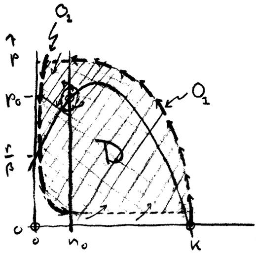
Construction of a "trapping region" (D) without equilibria, using two orbits ( $O_1$  and  $O_2$ ). The  $u \rightarrow$  unstable focus
