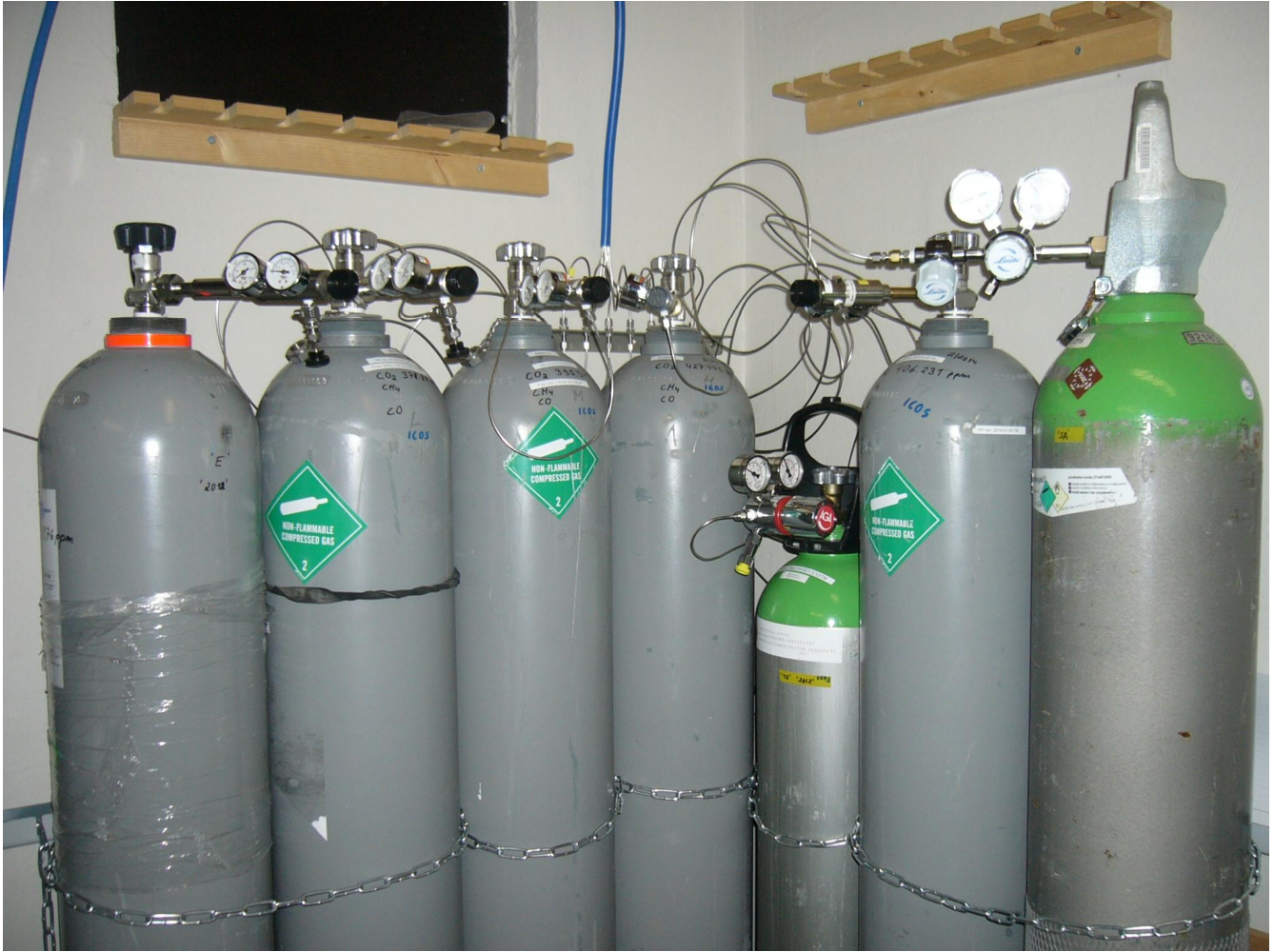
Figure 6. Calibration and target gas cylinders located in the main cabin basement.
