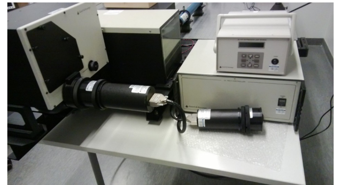
Integrating-sphere reflectance (or transmittance) spectrometer, from 0.250 \mu\text{m} to 3.2 \mu\text{m}
