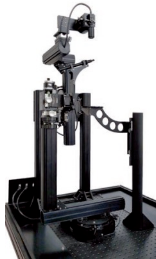
Spectropolarimetric goniometer for surface BRDF, from 0.420 \mu\text{m} to 0.9 \mu\text{m}
