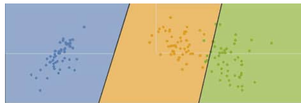
Figure 6.9: An example of a heuristic classification of the Iris data (after LDA transform) and the resulting areas of the variable space for the three classes.
