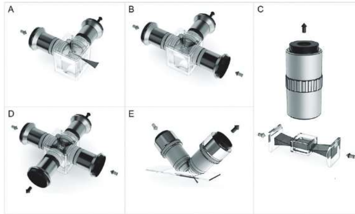
Figure 4. Implementations of light-sheet microscopy and benefits of multi-lens setups. Light-sheet microscopy is built around the sample and thus comes in numerous implementations. (A) A basic SPIM setup with one objective for illumination and one for detection. The sample is oriented vertically in the medium-filled chamber. (B) In this three-lens configuration, a second illumination objective is added for dual-side illumination. (C) An ultramicroscope with two illumination arms in an upright configuration with a low-magnification objective. The imaging chamber is typically isolated from the optical components to hold large, fixed samples in clearing agents. (D) A configuration with a second detection objective can be used to acquire images from two sides simultaneously for faster volume imaging. (E) A special objective configuration (iSPIM, diSPIM, Bessel and Lattice Light Sheet) for using cover-slip-mounted samples with light-sheet microscopy. Reprinted from Weber et al. Methods Cell Biol 2014;123:193–215, Copyright 2014, with permission from Elsevier
