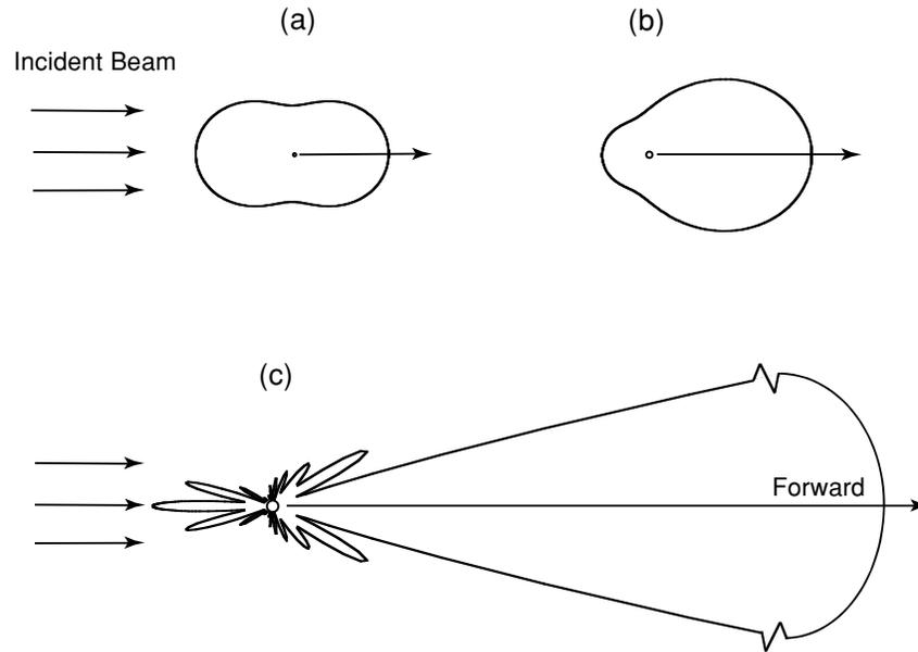
**Figure 1.4** Demonstrative angular patterns of the scattered intensity from spherical aerosols of three sizes illuminated by the visible light of  $0.5 \mu\text{m}$ : (a)  $10^{-4} \mu\text{m}$ , (b)  $0.1 \mu\text{m}$ , and (c)  $1 \mu\text{m}$ . The forward scattering pattern for the  $1 \mu\text{m}$  aerosol is extremely large and is scaled for presentation purposes.
