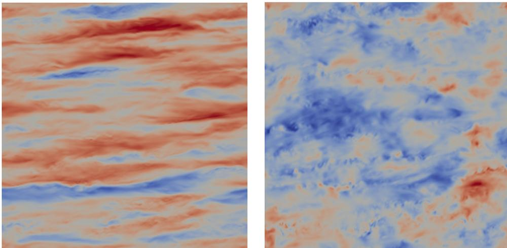
Figure 1. Instantaneous fields of horizontal streamwise velocity component (left) and vertical component (right).
